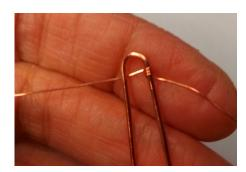
Using 26 gauge weaving wire, wrap approximatel 10 coil wraps around the frame.
